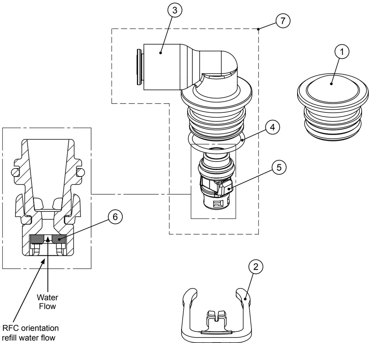
Proper RFC orientation directs refill water flow towards the washer face with rounded edge and text.
