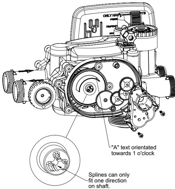
Noting the one possible orientation of the transfer drive cap, use one hand to press in and support the transfer drive cap while using the opposing hand to start two screws in, one on the top and one opposing it on the bottom. Tighten the screws in evenly so the cap seats the O-ring without getting pinched or damaged. Screws should only be hand tightened with a 5/32" or 4mm allen wrench, **DO NOT OVER TIGHTEN SCREWS.**
