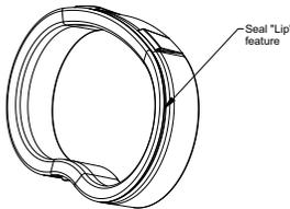
To remove seals gently pull out on the outer lip of the seal to lift the seal out from its cavity being careful not to damage the face surface of the seal. To reassemble re-seat seals into the seal cavity of the control valve body being sure that the lip of the seal is facing outward.
