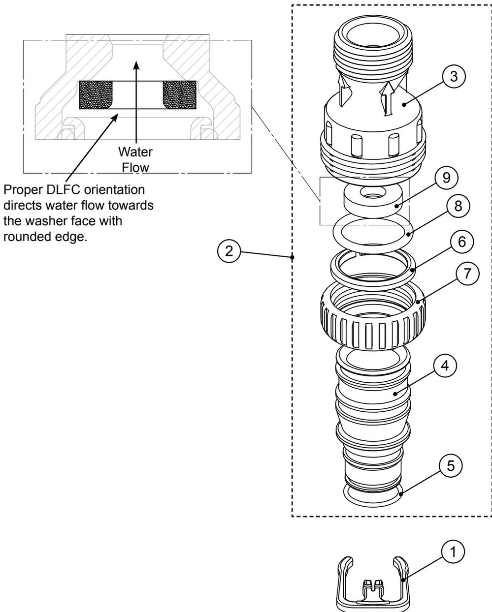
**V4017-01 TT Interconnect Fitting Assembly up to 10” tanks**
