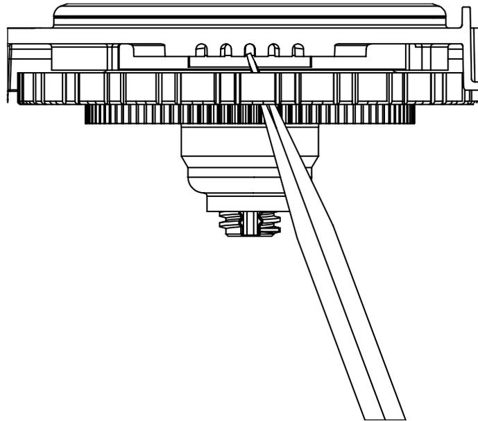
The drive cap assembly contains the drive cap, main drive gear, drive cap spline, piston rod, and various other parts that should not be disassembled in the field. The only replaceable part on the drive cap assembly is the O-ring. Attached to the drive cap assembly is the main piston (downflow or upflow) and, if a regenerant is used, a regenerant piston.
