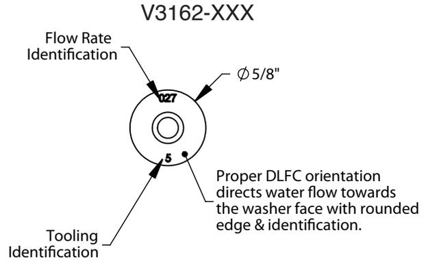
All DLFC housings ship without DLFC installed.
