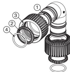
**Drain Line Flow Control Washers**
