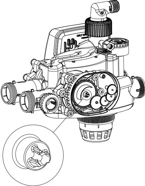
Position the large white drive gear with the A pointing toward the 1 o'clock position and then press it onto the stainless-steel drive shaft, make sure it snaps & locks into position.
