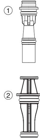
V3010-15B – V3010-15H injectors include one V3416 O-ring 012 (lower) and one V3171 O-ring 013 (upper).
